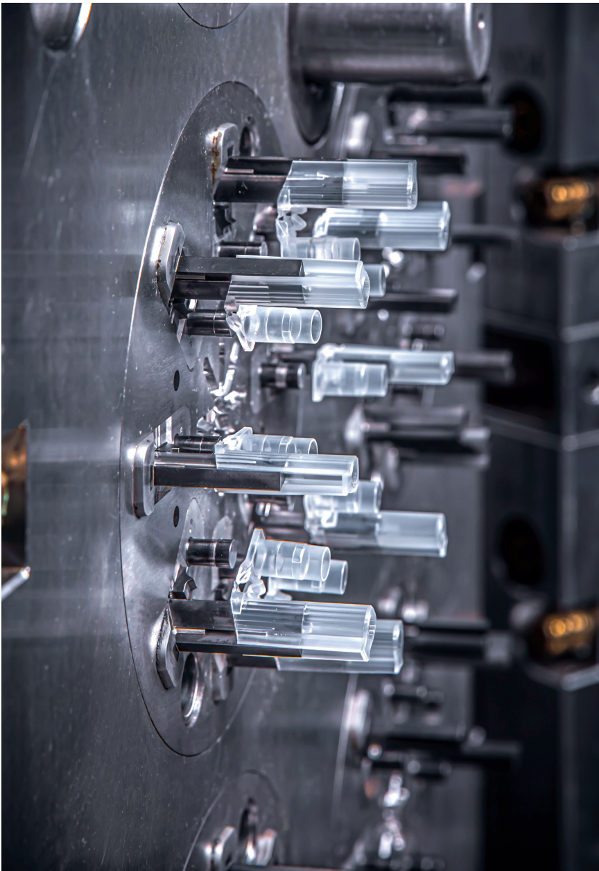
Partial automation of the demolding system represents an important step towards complete automation of injection mold design. © Werkzeugbau Ruhla
